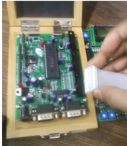
Fig. 7. Microcontroller training kit to design the Terminal Reader.
