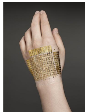
Fig. 6: Flexible electronics circuit develop at University of Tokyo [16]
