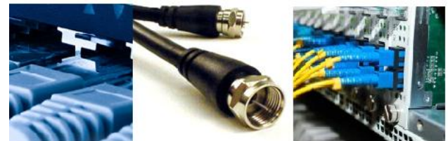
Fig 2: Cables (TP, Coax, FO)
