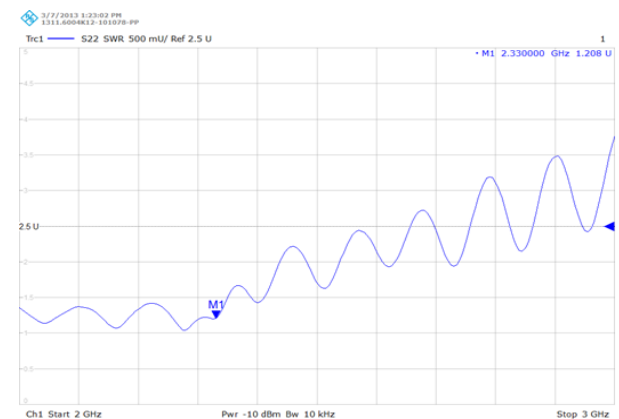
Figure 1. Voltage Standing Wave Ratio Vs Frequency Plot Experimentally
