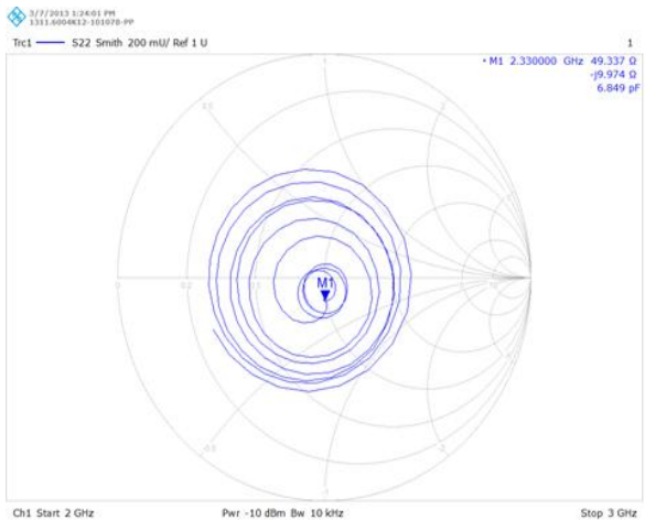
Figure 4. Voltage Standing Wave Ratio circles on Smith Chart Experimentally
