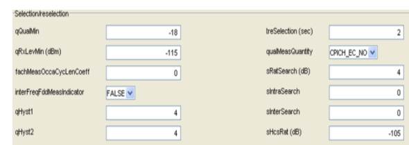
Fig 3: Parameters of handoff in idle mode
