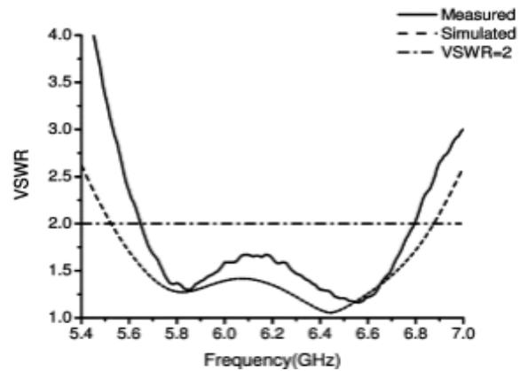
Fig.4. The simulated and measured VSWR.
