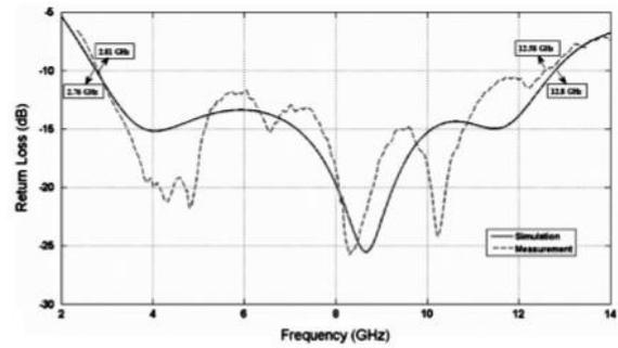
**Fig.7. Measured and simulated return loss of fabricated antenna**
