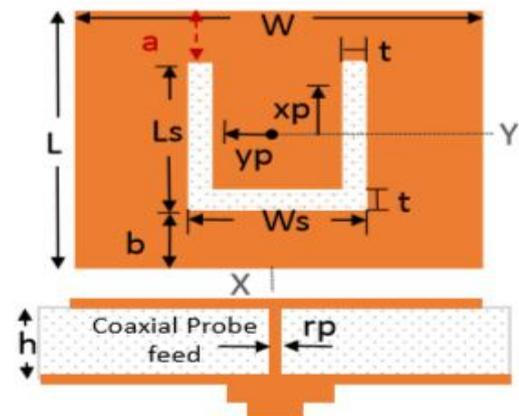
Fig.1. U-Slot loaded microstrip patch
