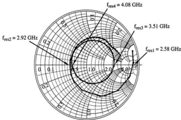
**Fig.6 Stimulated input Impedance of the initial U-slot microstrip patch used in the parametric studies. The four resonant frequencies of the structure are indicated**
