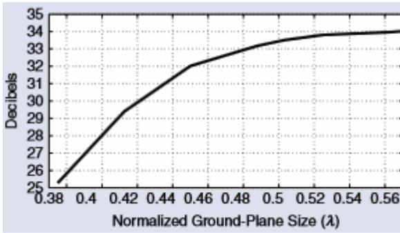
Fig. 9 The difference between the copolar and crosspolar levels versus the normalized ground-plane size
