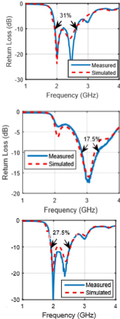
Fig. 2. Measured and simulated return loss on ( $r = 4.4$ ,  $h = 11.811$  mm) for (a) DIResF (b) DI (mod) (c) ResF (mod)
