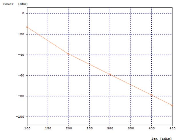
**Fig 4: Output optical power vs length for FWM component**
