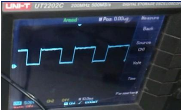
Figure10.PWMwaveof 100Hz on the digital oscilloscope.
