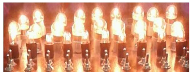
Figure16a.Less brightness on increasing PWM signal
