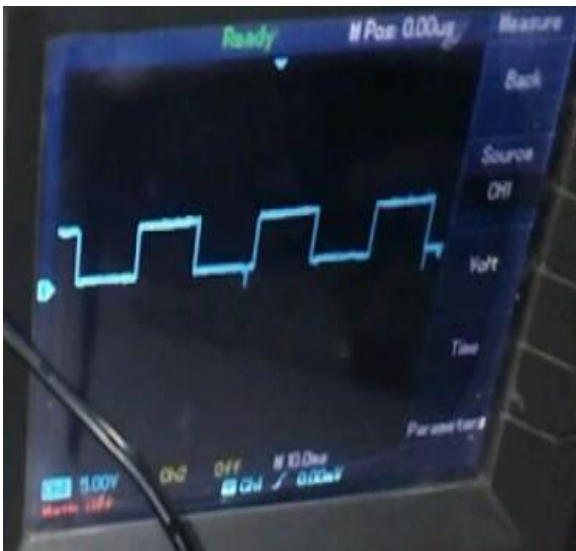
Figure11.PWM signal on the O/P of Mosfet.
